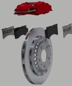
P-DEF plates have to be positioned between the brake lining and the caliper's pistons, creating a **barrier for the passage of the heat** given off during the braking. In this way, **Vapor-lock problems**, caused by the brake fluid as a consequence of an intense use of the brakes, are reduced.
