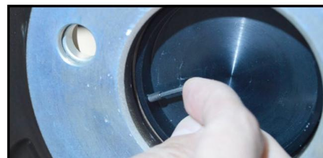
Fit the cap from the front face and fix the 3 small screws with the proper size 2 key.
