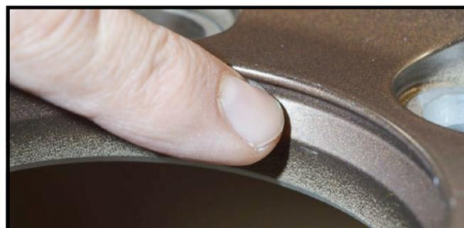
your wheel need to have a recess like this one, where the steel spring can expand and retain the cap.
