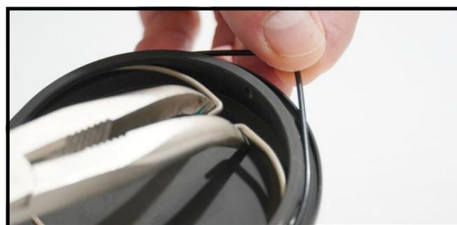
On the back of the cap there's a steel spring: you need to press it with the plier in order to shrink it inside the cap and fit it in the dedicated seat.
