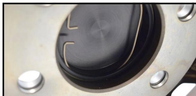
Mount the cap from the front face of the wheel, closing the spring with the plier and releasing it when the cap is in the proper position.
