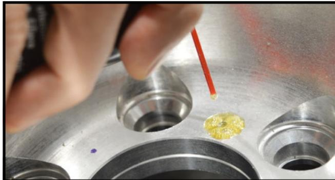
Use some cutting lubricant before proceeding with the threading operation.
