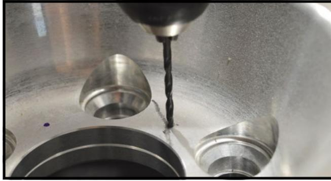
Drill the 5 holes with the provided tool HSS 3,3 mm diameter.
