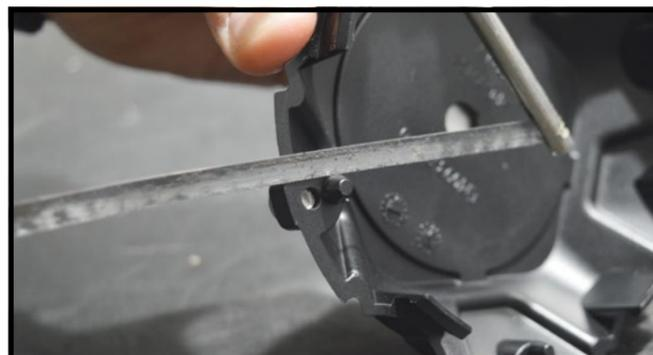
Cut the 5 round pins in correspondence of the screws holes: do not cut for the moment also the 5 clips as they may be useful to center the cap on the hub hole.
