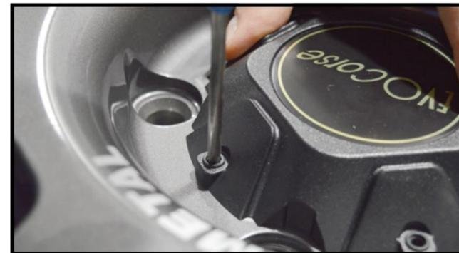
Use a sharp screw driver or a sharp pin to precisely mark the screw position: it is very important this is done carefully.
