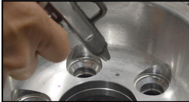
Blows away all the aluminum chips with some compressed air.
