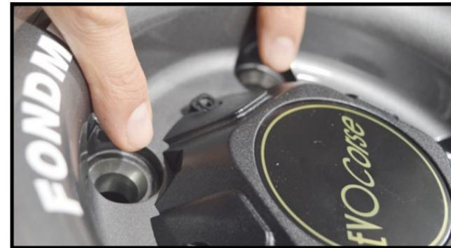
Fit the cap on the wheel, squeezing a bit the clip brackets: be sure it is well centered and that it is aligned with the nuts holes.
